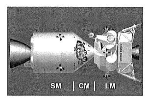
The Lunar Module was designed to hold two astronauts for the short trip between lunar orbit and the moon's surface. On the trip back to Earth, the astronauts were required to spend more time than expected in the lunar module.
